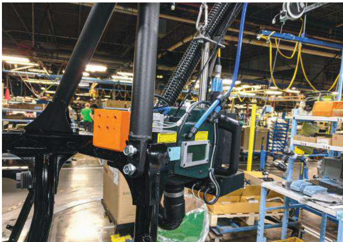
Kawasaki’s laser engraving system etches vehicle identifications numbers (VIN) onto vehicle frames with a 3D printed clamp (left).
