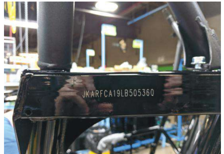
Kawasaki’s laser engraving system etches vehicle identifications numbers (VIN) onto vehicle frames with a 3D printed clamp (left).
