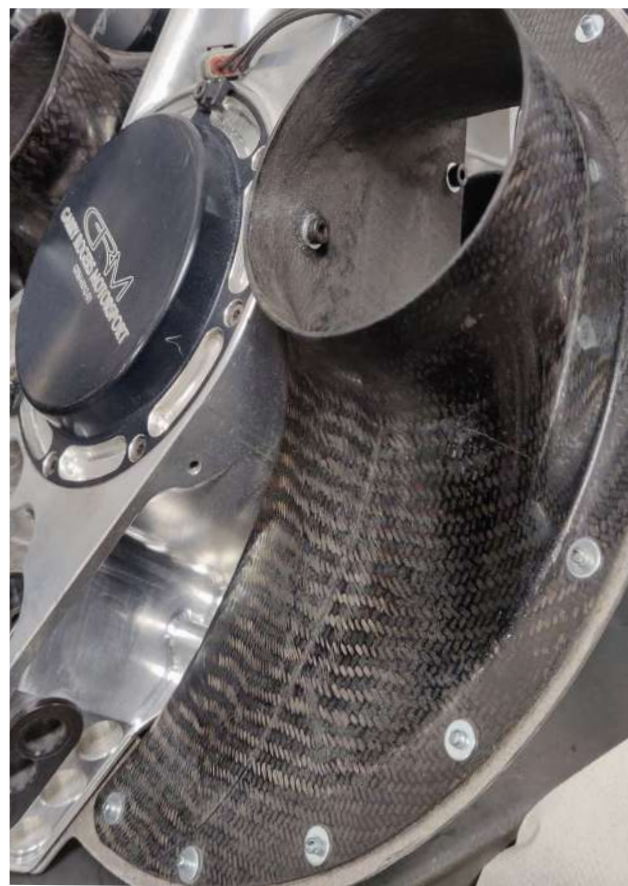
The final brake duct, which was made using a 3D printed brake duct pattern.
